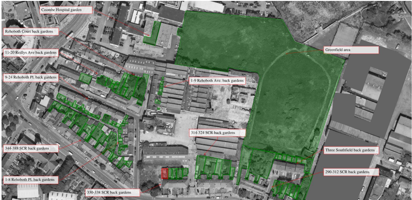
Figure 3: Diagram showing the location of surrounding amenity spaces tested and the relative impact. Areas in green will experience a negligible impact. The area shown in red will experience a reduction outside of the BR 209 (2022) guidelines.
